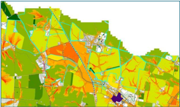
Figure 4. Water flow across fields (orange/red ‘flashes’) and how connected fields are to a watercourse (green = least connected, through to yellow and orange, and dark orange/red = most connected).
