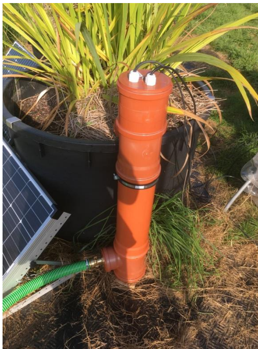
Fig. 9: Multiparameter sensor in the inflow pipe
