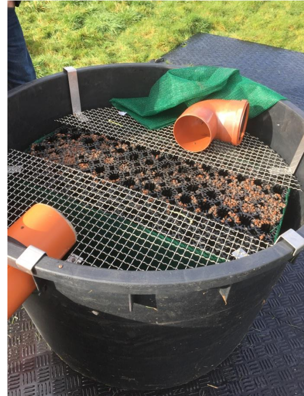
Fig. 8: Plastic carriers and burnt clay inside one wetland pot
