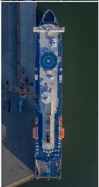
Scandlines ferry, MV Copenhagen made port in Rostock to be transformed overnight into a wind-assist hybrid vessel. The installation of the large 30m tall Rotor Sail supplied by the Finnish company Norsepower Oy Ltd took only a few hours meaning that the ferry was ready for operations the next morning, and this installation is expected to reduce emissions by an estimated 4-5 percent.
