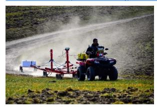
Driven by the need for more effective tools to describe groundwater/surface interaction, raw material, point source pollution and other geotechnical applications, in all TOPSOIL countries, tTEM¹ surveys have been planned. Due to Corona, the implementation of the surveys has been delayed. However, the time has been used to further improve and develop the system.
