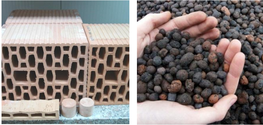
Figure 4.11. Thermal immobilization combined with the production of bricks or light weight aggregates [Ref. 23]
