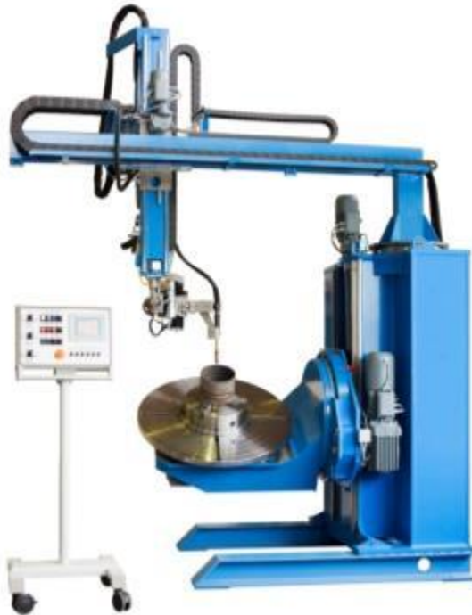
Automatic multi-axis for 1 ton positioner for the MIG-MAG welding of valves
