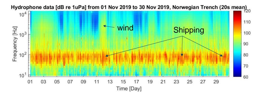
Shipping dominate the ambient noise between 20 and 500 Hz, while noise from wind and waves dominate over 1000 Hz.
