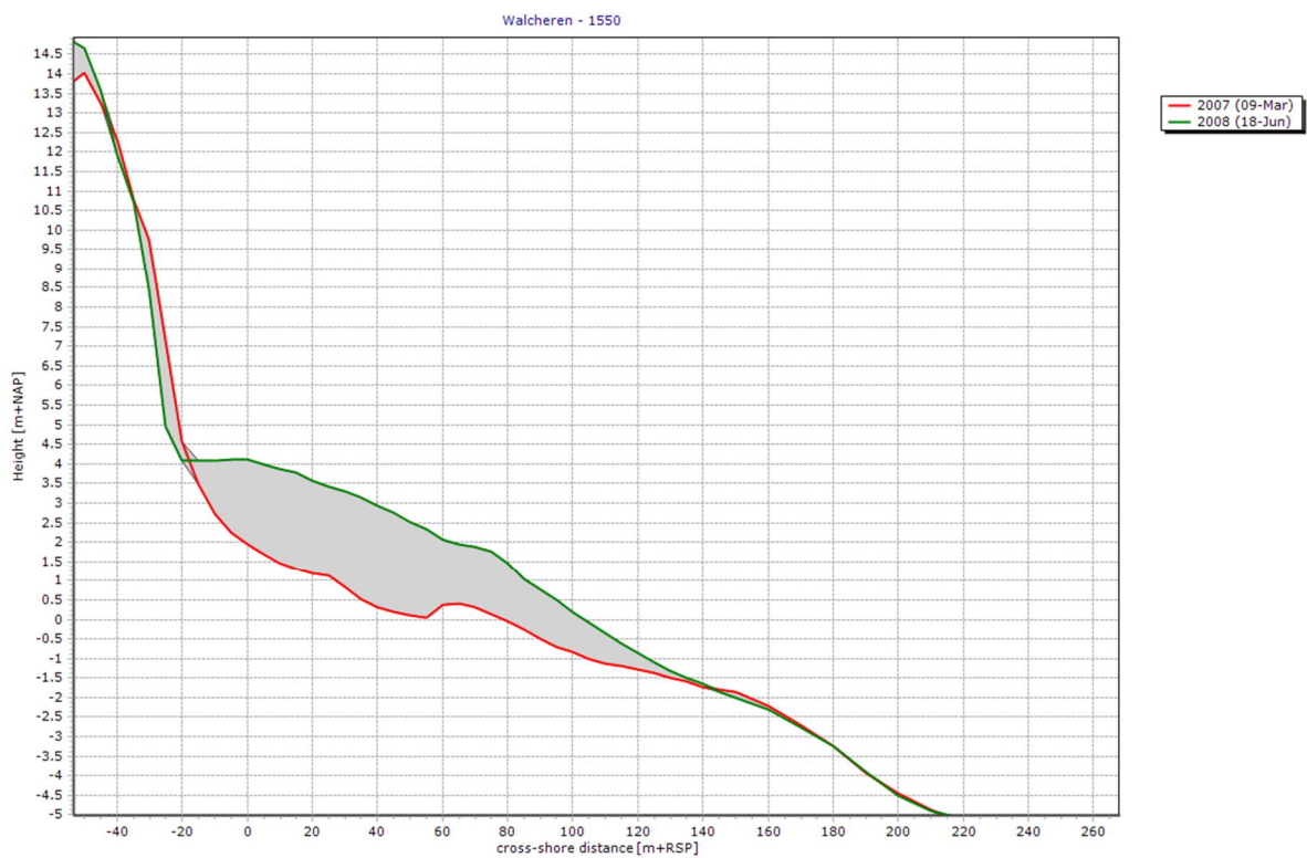
Figure 8: Placement of nourishment in transect 1550
