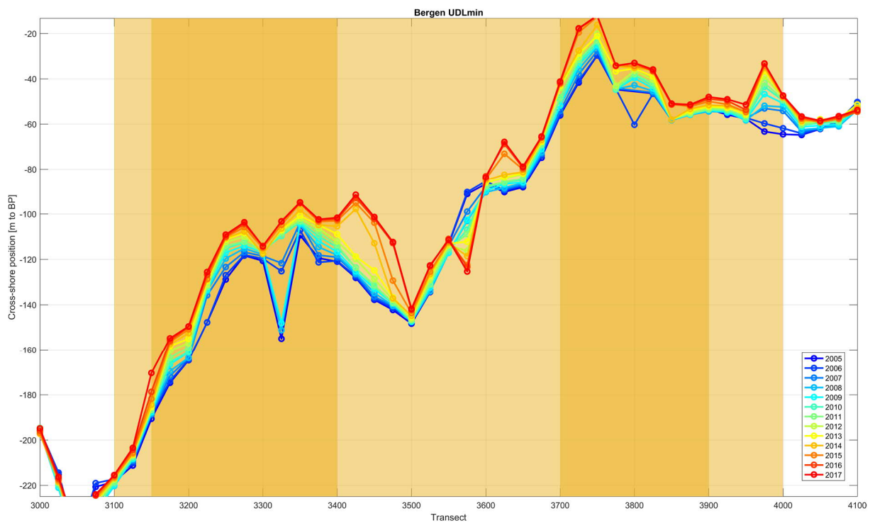
Figure 50: Position of the upper dune level for the transects in the study area (3000 is in the north, 4100 in the south) from 2005 to 2017. Squares indicate nourishment positions: shoreface nourishment (yellow) and two parts of the beach nourishment (orange).
