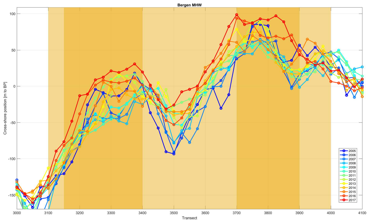
Figure 53: Position of the mean high water line for the transects in the study area (3000 is in the north, 4100 in the south) from 2005 to 2017. Squares indicate nourishment positions: shoreface nourishment (yellow) and two parts of the beach nourishment (orange).
