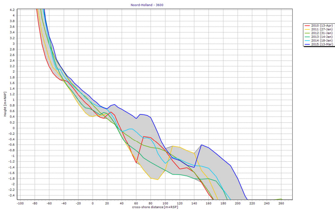
Figure 37: Profile 3600 showing the zone around the beach in between the northern and southern beach nourishments
