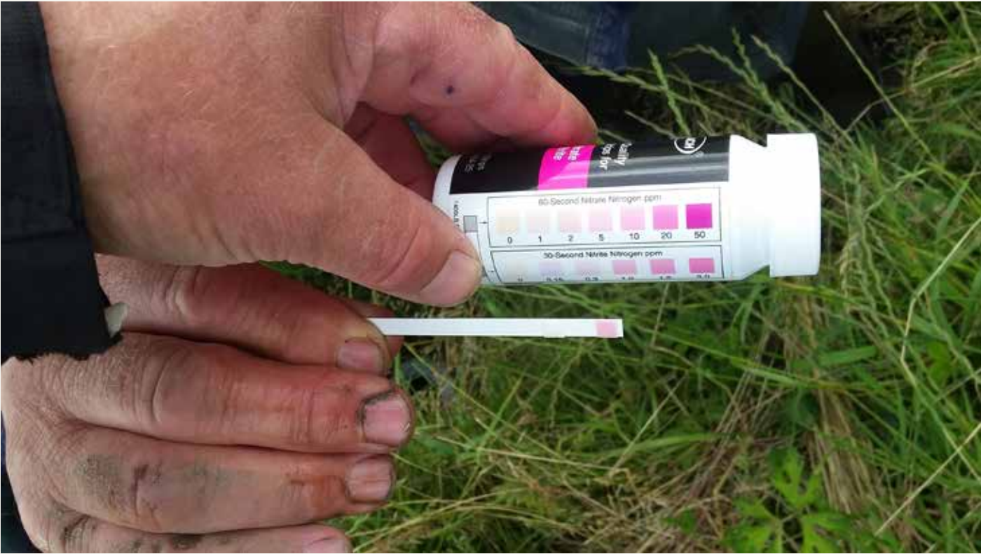
Test strips are practical for deciding levels of nitrate concentration.
