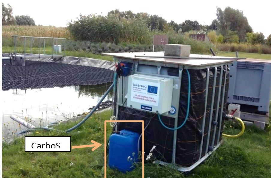
Photo 3 Moving Bed Biofilm Reactor at PCS in 2019 with CarboST as C-source
