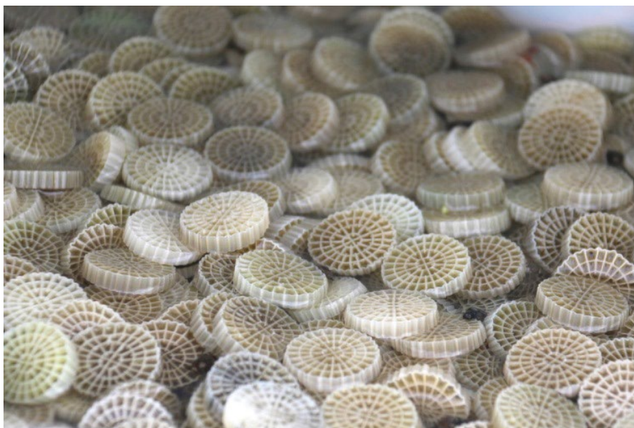
Photo 1 Plastic carriers in a MBBR, on which a biofilm will develop
