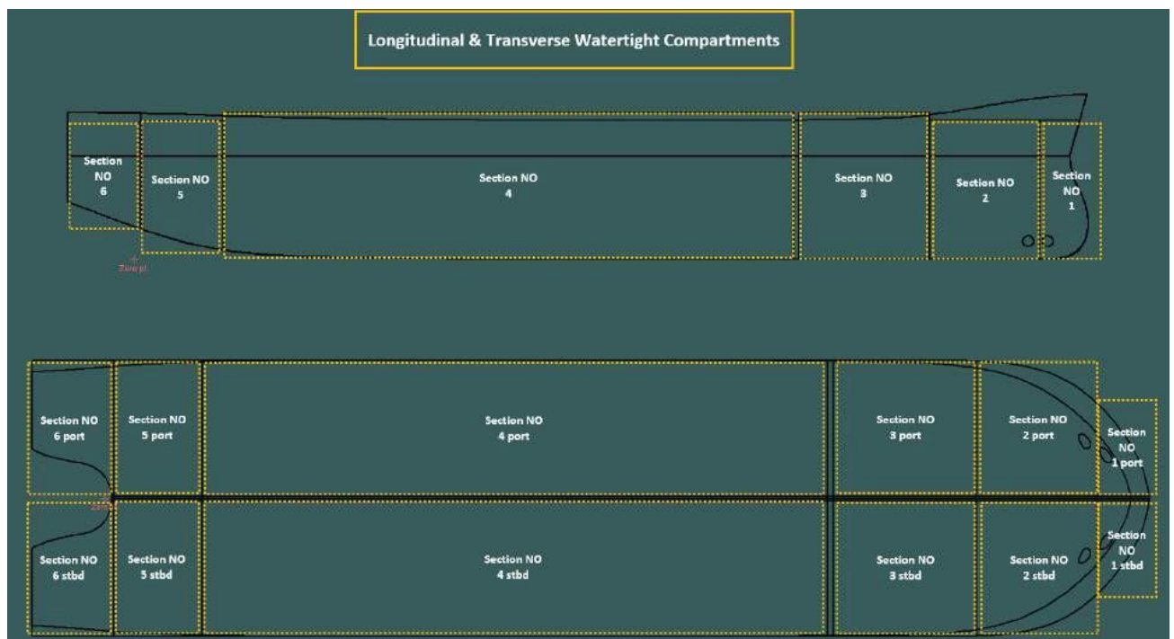
Figure 5-18 Longitudinal and Transverse Watertight Compartment
