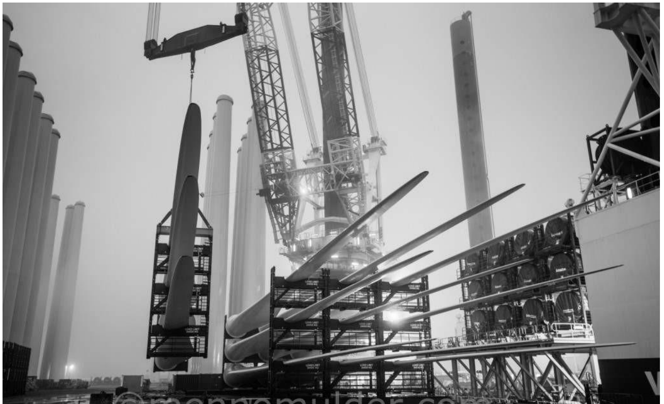
Figure 3-32 Load Out of Turbine Blades onto the Vole au Vent Jack up Vessel (Mulder 2019)
