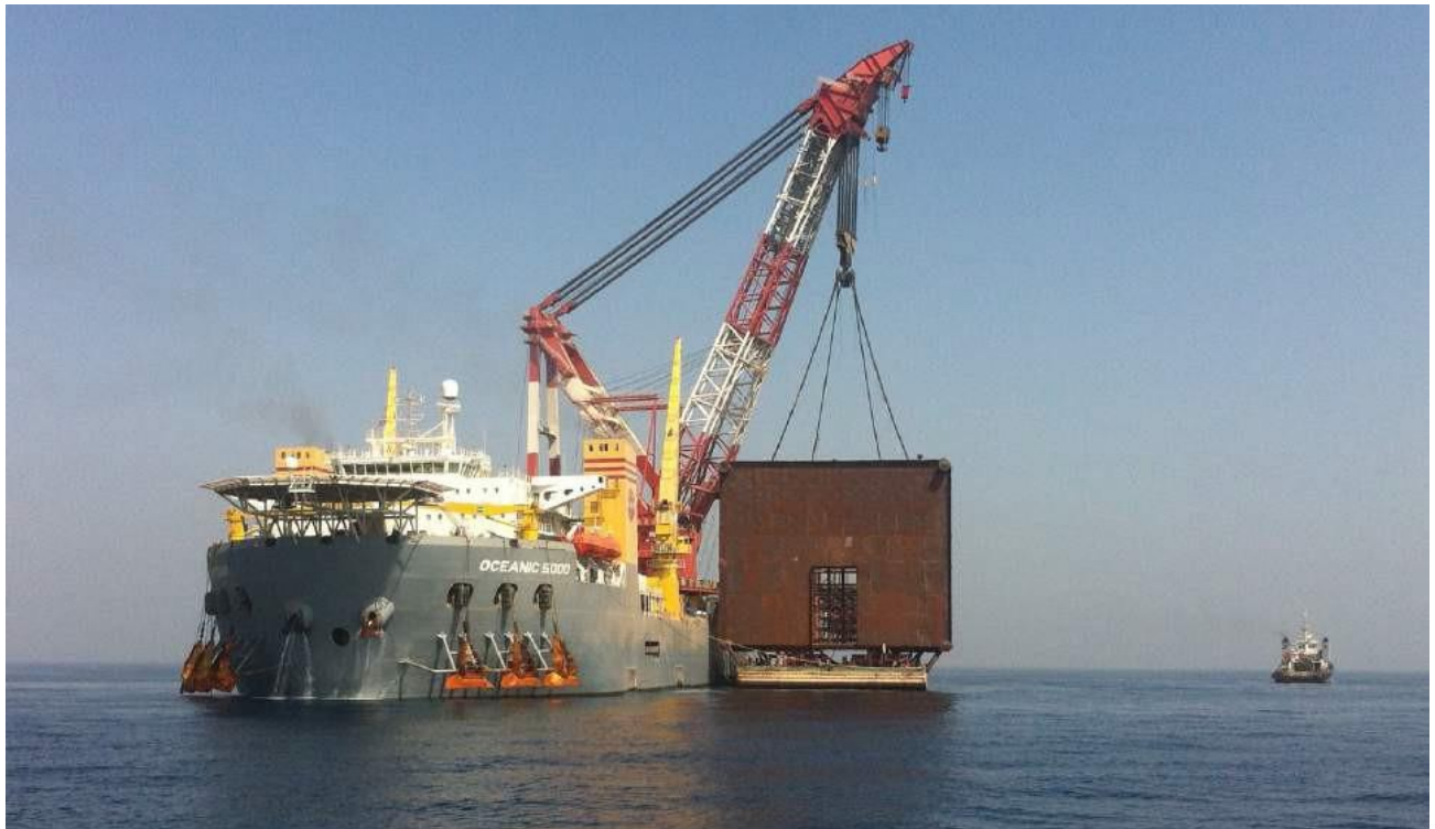
Figure 3-2 The Jacket is loaded onto the C/V and Tied up to the HLV
