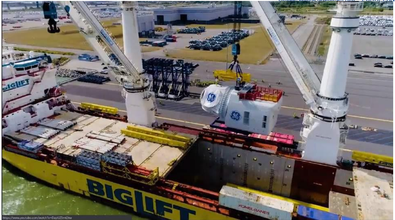
Figure 6-9 Lifting 12MW GE X-Heliade Nacelle into the C/V (Pondera 2019)
