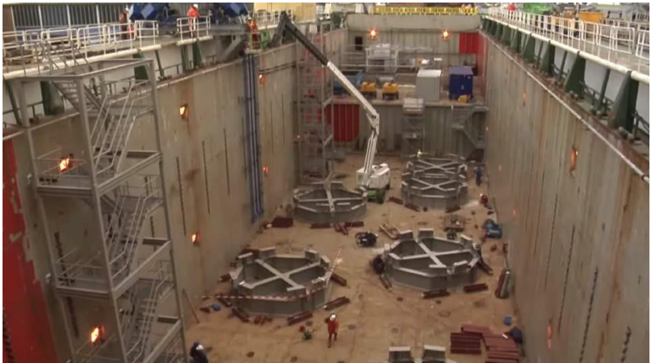
Figure 6-56 Seafastening of TP inside the vessel holds (Jumbo Maritime 2010)
