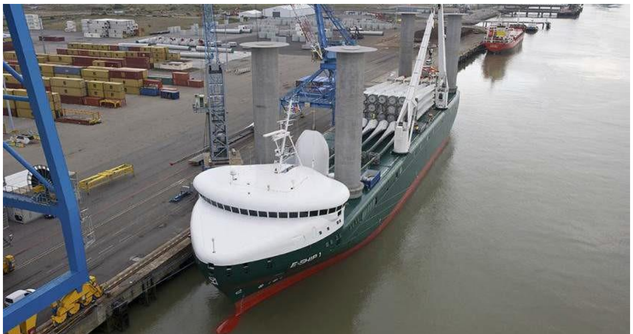
Figure 5-48 Enercon E-Ship 1 (equipped with 4 number of Flettner rotors)
