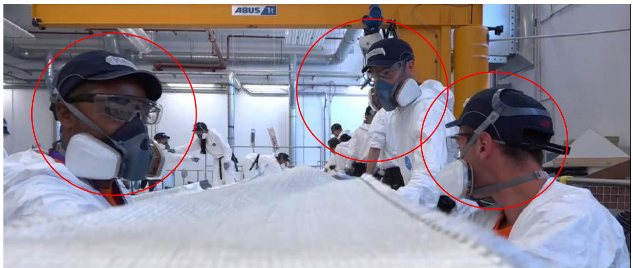
Figure 6-72 Manufacturing of 12 MW Blade (all staffs with Special Face Mask and PPE)
