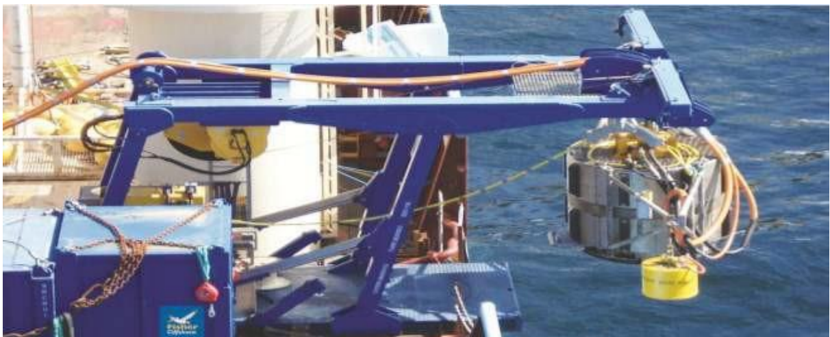
Figure 6-205 LARS of Mass flow excavator (James Fisher and Sons 2014)
