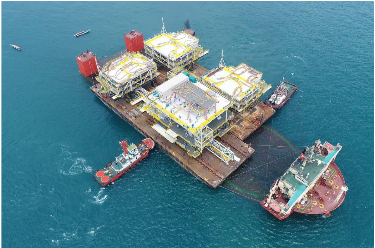
Figure 3-13 Heavy Load Carrier During Loading 4 Topsides which are loaded on 2 Barge (SAL n.d.)
