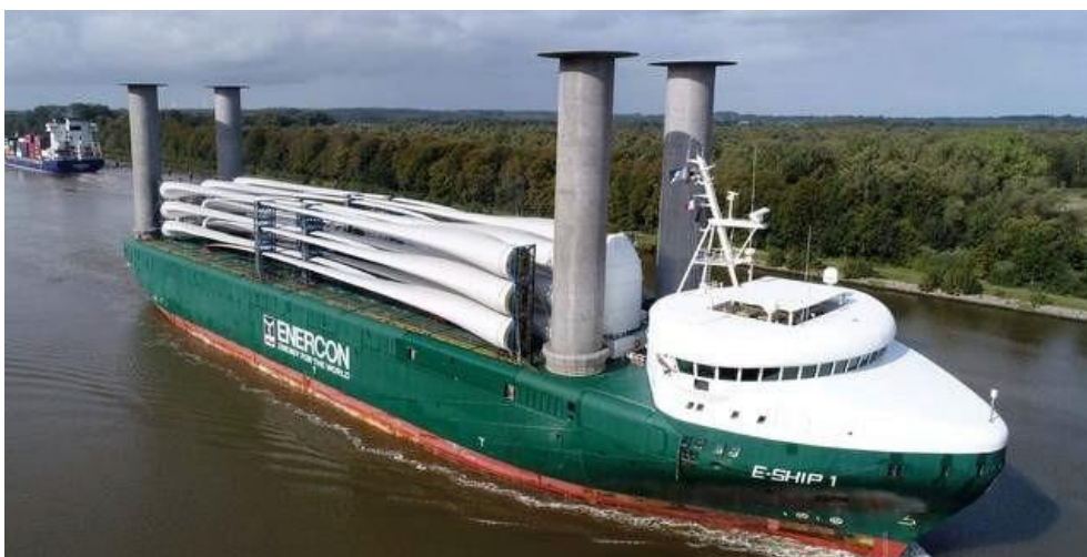
Figure 4-29 Enercon E-Ship 1 is Equipped with 4 Rotors 41
