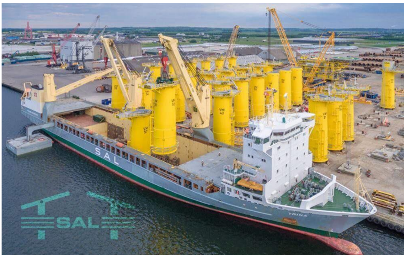
Figure 3-14 SAL Trina Loading Transition Pieces
