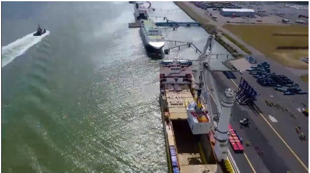
Figure 6-10 Lifting 12MW GE X-Heliade Nacelle into the C/V (Pondera 2019)
