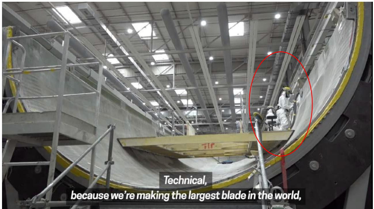
Figure 6-71 Manufacturing of 12 MW Blade (all staffs with Special Face Mask and PPE)
