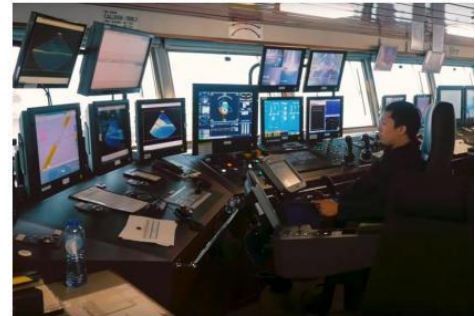
Figure 5 Seatools has an extensive track record in ROV automation. Like our fall pipe ROVs, the Carrera E comes with a large degree of process and navigational automation. Thanks to these ROVs high degree of automation, a complete ROV system, can be operated by a single operator.
