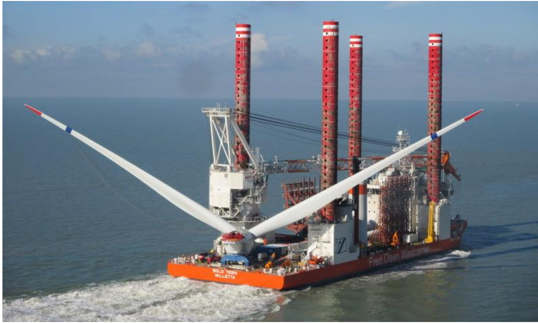
Figure 27 Transportation of nacelle and blades with bunny ear configuration (International Cranes, 2013)
