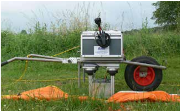
A smaller seismic source called "ELVIS"
