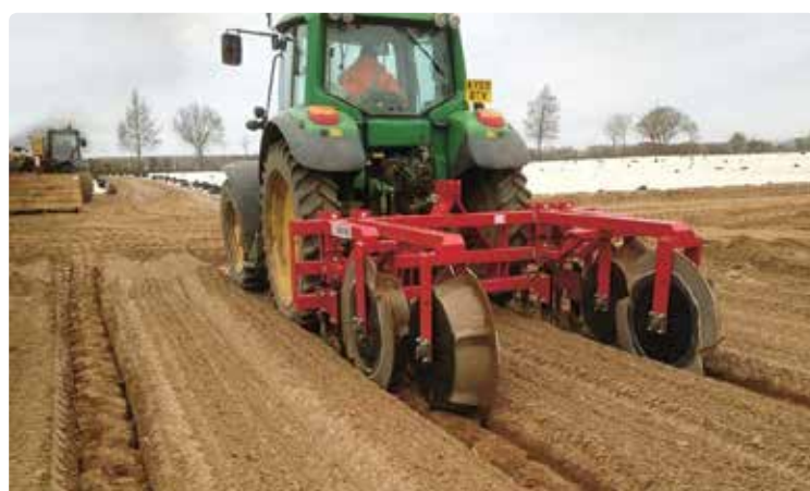
Tramline disruption technology being trialled in a potato crop on the Elveden Estate, UK.
