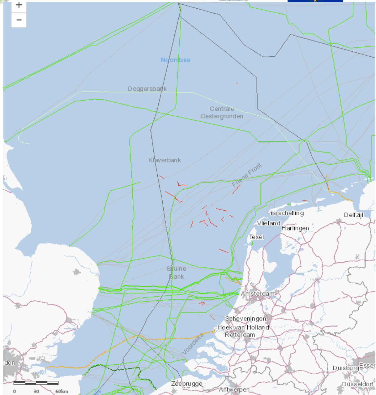
Figure 7. Map of cables in the Netherlands marine area showing electricity cables (orange), telecom cables (green) and export cables (red). Source: North Sea Atlas
